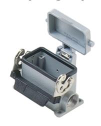
Surface mounting housing, C-TYPE series, with 1 lever, M40 cable entry, size "57.27", high construction, with metal cover
