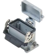
Surface mounting housing, C-TYPE series, with 1 lever, Pg29 x 2 cable entry, size "57.27", high construction, with metal cover
