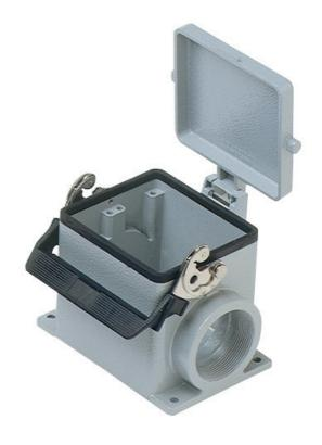
Surface mounting housing, C-TYPE series, with 1 lever, M40 cable entry, size "77.62", with metal cover
