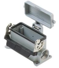
Surface mounting housing, C-TYPE series, with 1 lever, M25 x 2 cable entry, size "77.27", with metal cover
