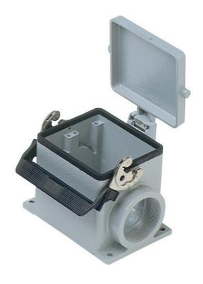
Surface mounting housing, C-TYPE series, with 1 lever, M50 x 2 cable entry, size "77.62", with metal cover
